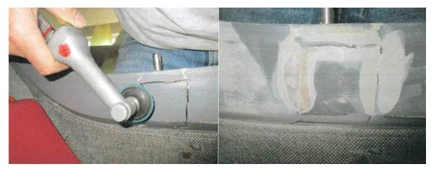
• by use of sanding paper or a sanding machine remove the paint on the inner canopy frame at the damaged spigot until the contour of the cover plate becomes visible
